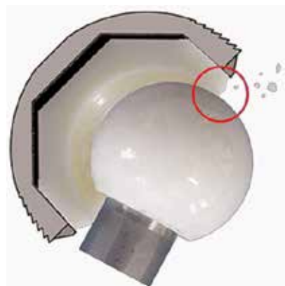
Loss of congruence, concentration of loading at a single point and risk of breaking
