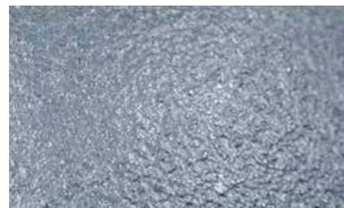
Ti6Al4V with porous titanium coating, magnified
