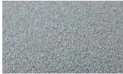
Ti6Al4V with HA Coating, magnified
