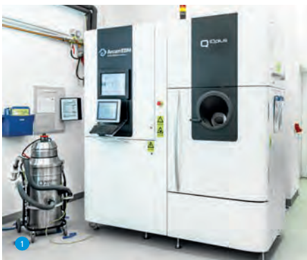
LINK has several of these innovative systems for additive manufacturing (1). At the end of the production process, the powdery »cake« is removed from the machine (2). The freshly manufactured implants are exposed in a special blasting cabin (3). Top: Compilation of LINK products made by additive manufacturing.
