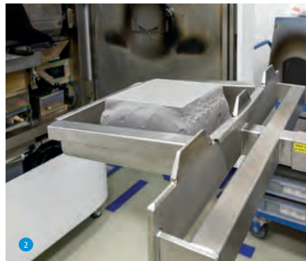
LINK has several of these innovative systems for additive manufacturing (1). At the end of the production process, the powdery »cake« is removed from the machine (2). The freshly manufactured implants are exposed in a special blasting cabin (3). Top: Compilation of LINK products made by additive manufacturing.
