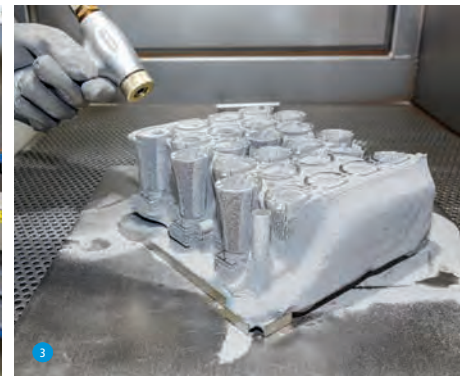
LINK has several of these innovative systems for additive manufacturing (1). At the end of the production process, the powdery »cake« is removed from the machine (2). The freshly manufactured implants are exposed in a special blasting cabin (3). Top: Compilation of LINK products made by additive manufacturing.
